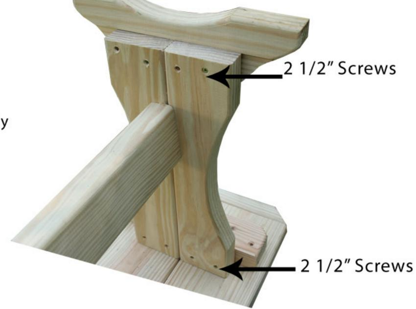
**Step 3.** Step 3. Place the 2x4 spreader between the leg assemblies. (Having a second person to help you makes this step easier.) Attach the 2x4 spreader to the leg assembly by lining up the spreader with the pre-drilled holes in the leg assemblies. Attach the 2x4 spreader by using four (4) 2 ½" screws. Two per side.
